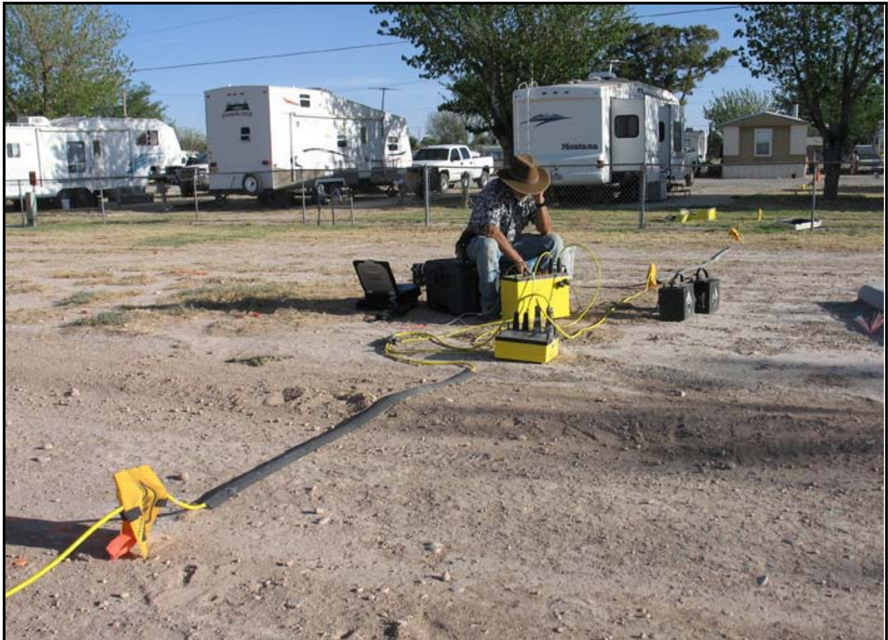
Lewis Land conducting electrical resistivity survey of the I&W brine well cavity in Carlsbad; Stop 1 of the Evaporite Karst field trip. Photo by NCKRI.
