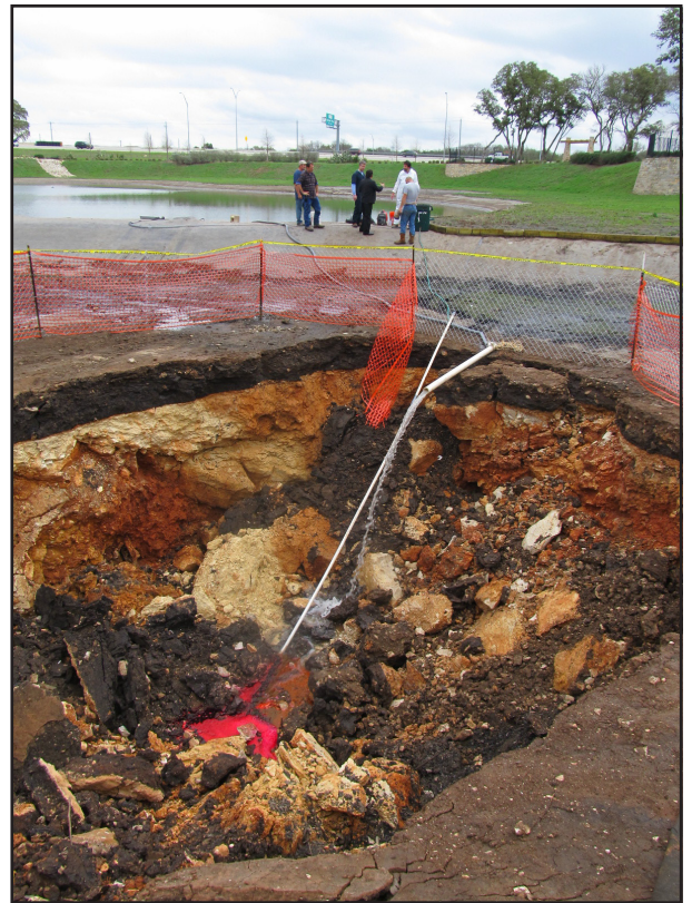
Dye tracing performed in a sinkhole collapsed within a storm water retention pond on the Edwards Aquifer of central Texas. Photo by Brian Hunt (BSEACD).
